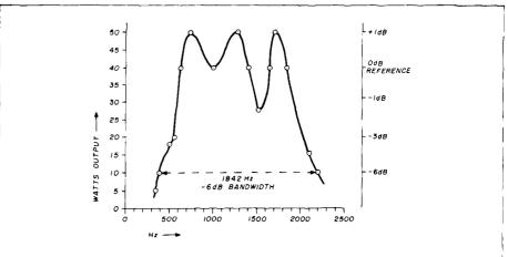
fig. 7. Passband of Collins KWM-1 transceiver with F-455N-20 filter. Note the "notch" at about 1500 Hz.
